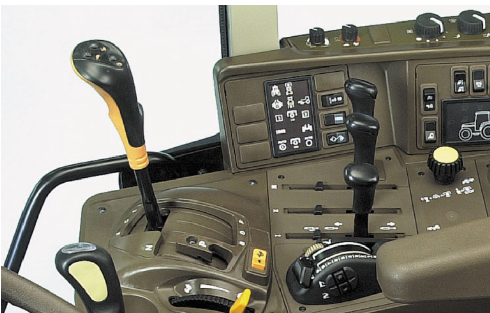
Figure 2: Range lever with two push buttons to power- shift gears (above) and the resume switch to activate the automatic shifting system (below, middle)
